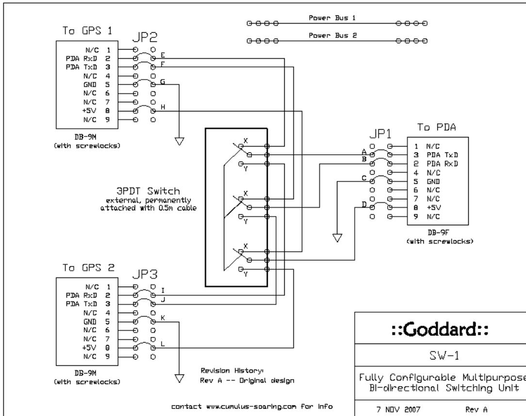
As you can see, with the existing 'as shipped' condition, the switching unit allow you to switch pins 2, 3, and 8 from two separate units on the left to the corresponding pins on the right.
