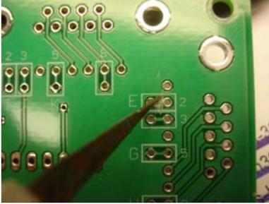
Using a razor or Xacto knife, cut through the desired trace interrupting the connection.
