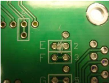
Be sure that the trace is completely broken by checking with a multimeter for continuity.
